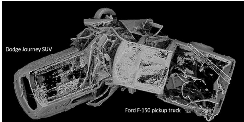
Figure 9. Approximate orientation of vehicles at maximum engagement during crash.
